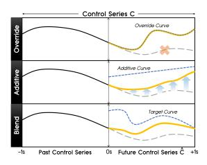
Fig. 5. Override, additive, blending layering of multiple control series.
