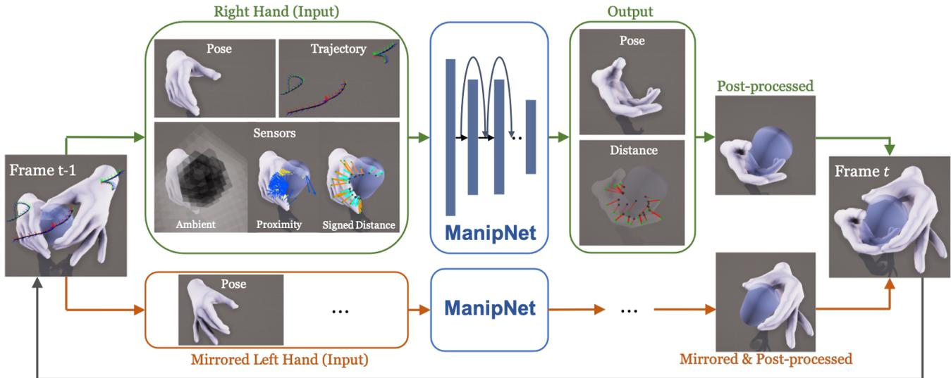
Fig. 2. The outline of our framework. Given the poses of two hands, the shapes of objects as well as the trajectories of two wrists and objects at frame  $t - 1$ . The inputs of the two hands will be generated separately and fed into a shared neural network. Correspondingly, the poses for the two hands at frame  $t$  will be synthesized from the outputs of the neural network.
