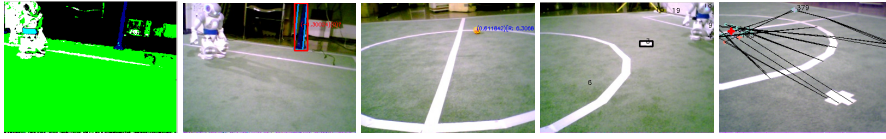
Fig. 2. Representative output of the Vision module - real time detection of key features based on colour segmentation.
