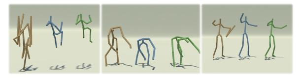
**Figure 1:** A set of corrupted motions (orange) fixed by projection onto the motion manifold (blue) and compared to the ground truth (green). Motion corrupted with artificial noise that randomly sets values to zero with a probability of 0.5 (left), motion data from Kinect motion capture system (center), and motion data with missing the wrist marker (right).
