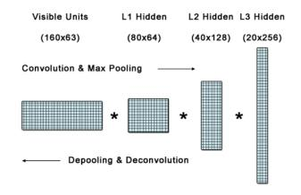
**Figure 3:** Units of the Convolutional Autoencoder. The input to layer 1 is a window of 160 frames of 63 degrees of freedom. After the first convolution and max pooling this becomes a window of 80 with 64 degrees of freedom. After layer 2 it becomes 40 by 128, and after layer 3 it becomes 20 by 256.
